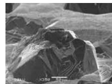
Controlled breakdown with self-sharpening effect
