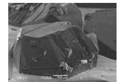
Grains are wearing flat, increasing the contact area
