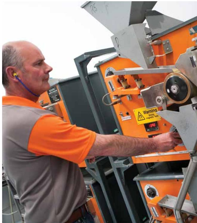
At the Element Six Micron+ Production Centre the incoming synthetic diamond is magnetically separated, milled to shape and size. The micron is then cleaned and rinsed before sedimentation.
